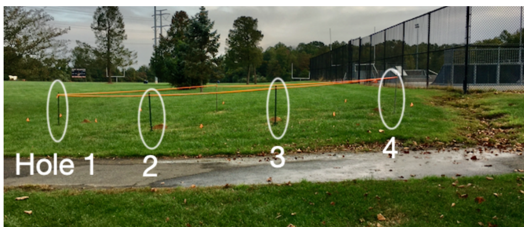
Figure 13: Infiltration test holes
